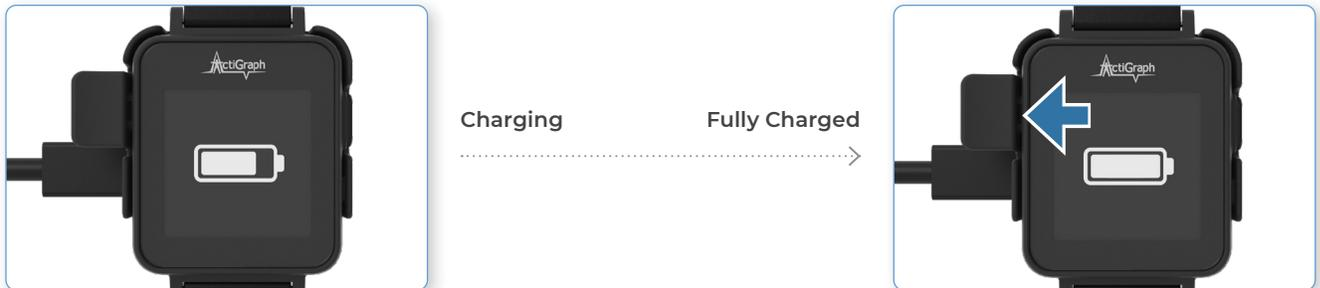
3. Remove the CPW01 from the charging dock by pulling the plastic tab to the left and away from the CPW01. Continue wearing the CPW01 according to instructions.
