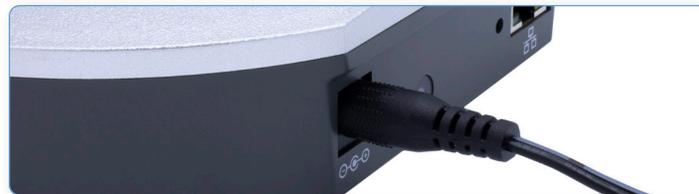
3. The blue LED on the back of the CP Data Hub will begin to flash during startup. Once the CP Data Hub connects to the cellular network, the blue LED will stay on solid.
